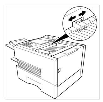
Pull the blue Pressure Adjusting Lever upward and slide it to the desired position depending on the condition.
